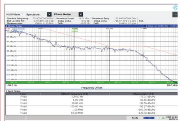
▲ Fig. 8 Measured phase noise at 52.4 GHz.
