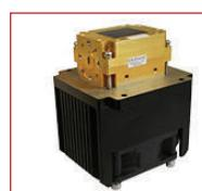
Model SBP-4036033436-1919-EP offers 34 dB small-signal gain over the 40 to 60 GHz frequency range and +36 dBm saturated output power. The amplifier features WR-19 waveguide input/output with anti-cocking UG-383/U-M flanges and operates from a
