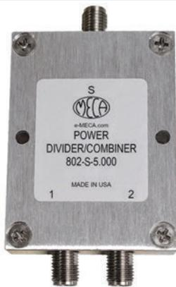
**M**ECA Electronics' new 802-S-5.000 broadband power divider operates across 2.00 to 8.00 GHz frequencies, spanning the needs of S- and C-Bands and Wi-Fi 6E through Wi-Fi 8. This two-way power divider uses a Wilkinson configuration with SMA connectors. The 802-S-5.000 delivers an amplitude balance of 0.3 dB and phase balance of 4 degrees, performance previously challenging to find outside of narrowband products.
