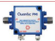
PMI Model P1T-DC18-60-T-SFF-HSLVT is a single pole, single throw, absorptive switch that offers ultra-low video transient performance while providing ultra-fast switching speed of 6 ns; high isolation of 60 dB min. to 12 GHz, 70 dB min. to 18 GHz; and 4.5 dB max. insertion loss. This switch module contains an integral TTL driver and the DC supply voltage is only -5 VDC. Includes SMA female connectors in a housing that measures 1.0 x 1.0 x 0.5 in.
