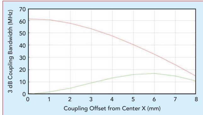
▲ **Fig. 3** 3 dB coupling bandwidth of dual-post modes according to the configuration in Figure 2: red – basic mode (at 2.23 GHz), green – second mode (at 2.77 GHz).
