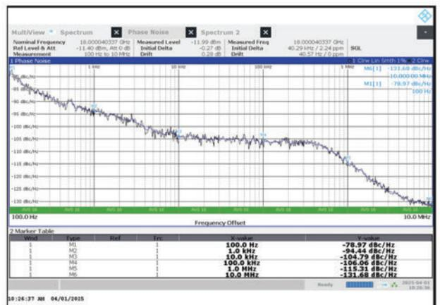
▲ Fig. 7 Measured phase noise at 18 GHz.
