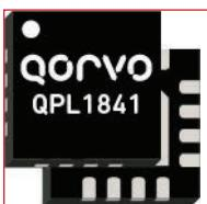
The QPL1841 is a GaAs pHEMT single-ended MMIC RF amplifier IC featuring 12 dB of gain and low noise from 5 to 850 MHz.
