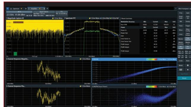
▲ Fig. 4 Screenshot from FSWX showing dual-channel measurement of amplifier input and output.
