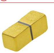
Knowles' Milli-Cap® broadband blocking capacitors are designed to minimize parasitics and deliver stable, low loss performance across wide frequency ranges. Their ultra-high series resonance and very low inductance make them ideal for demanding RF applications like test equipment, fiber-optic modules and broadband
